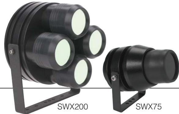
Choose from three types of filters to suit your specific application: overt illumination produces a distinct red glow that warns of the presence of IR light (715 nm), semi covert illumination produces a faint red glow that can be detected with a trained eye (850 nm) and full covert illumination avoids any red glow, making it impossible to detect the presence of IR light (950 nm)
