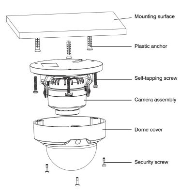
4. If you are flush mounting the camera and want to store the cables inside the wall or ceiling, drill a hole at the cable exit position on the mounting template and then pull the power and video cables through the hole.
